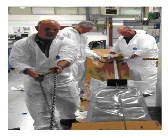
Shane pulling the wetted out carbon unis for the 35 mm diameter solid carbon wing joiner. It took a 1.5 ton chain block to pull them through the aluminium forming tube and fire extinguisher to cool!
