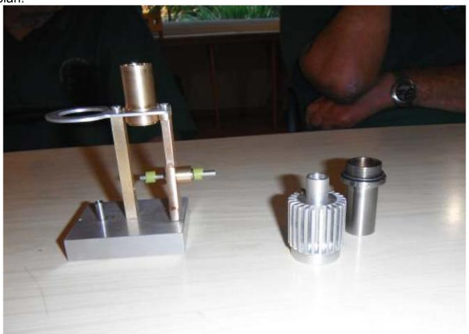
Ken McIntyre showed the small project he is currently working on - a miniature ring bottom hot air engine. This is very light in construction
